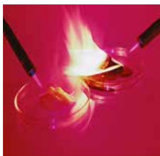
Hydrocarbon-based lubricants burn; Krytox™ does not.
